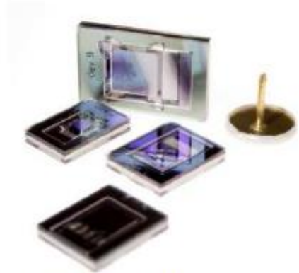
Elfrink et al., 2008, IMEC 60 \mu\text{W} , 2g @ 572Hz, 0.2 \text{cm}^2
